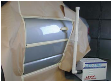
Air Tubes can be set up any way you like, or make your own with Standard PVC Pipe.
